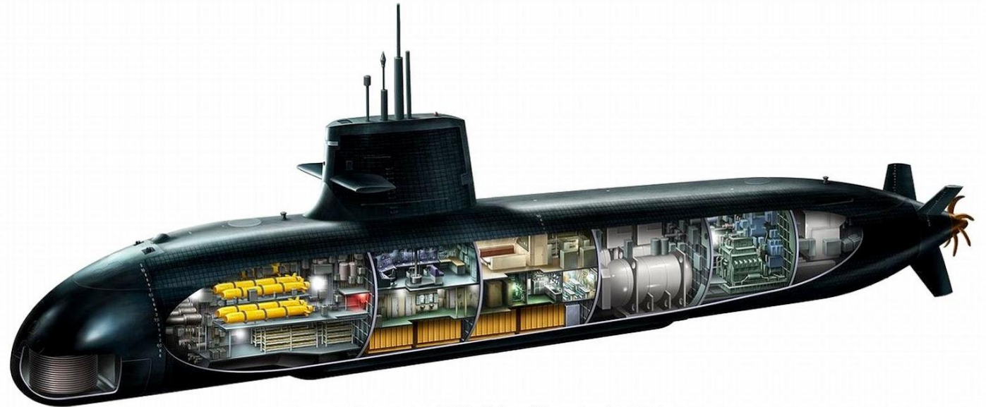
AIP Stirling Engines Soryu class submarine SS-501 ~ SS-510
