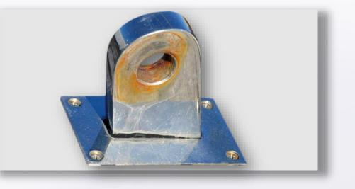
It originates in confined spaces where corrosive products become trapped, retaining ions and generating variations in oxygen concentration. Bolted joints, gaskets, and flanges are common sources of this type of corrosion.
